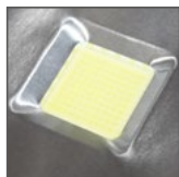
dioda LED typ COB (Chip on Board)
