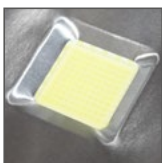
dioda LED typ COB (Chip on Board)
