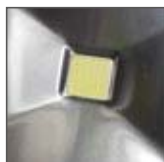
dioda typu COB (Chip on Board)
