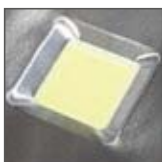
dioda LED typ COB (Chip on Board)
