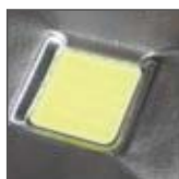
dioda LED typ COB (Chip on Board)
